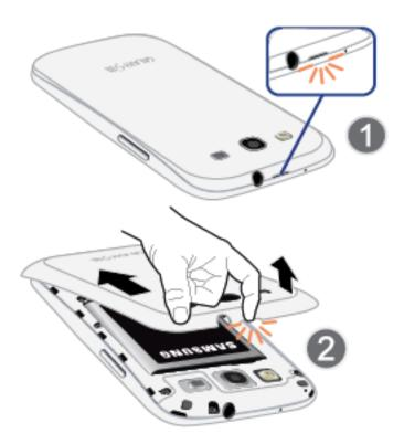
Insert the battery, contacts end first, and gently press the battery into place.
