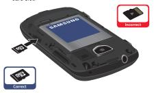
2. Push the microSD card into the slot until it locks into place.
