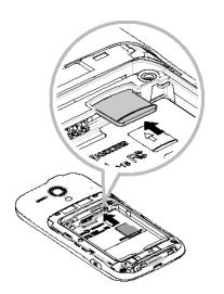
4. Replace the battery and the battery cover. See Insert and Charge the Battery.
