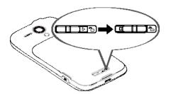
Insert your thumbnail or fingernail into the slot and lift the battery cover gently.
